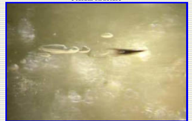
Inclusions of gas bubbles and a drop of dark glass. The elongated shape of the inclusions indicates a flow of the glassy mass in the gel state. Source: Richard de Nul
